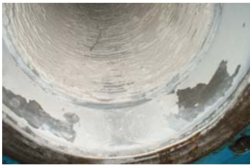
Crystallisation of fluids when they get in contact with oxygen can deform and damage the plates.
