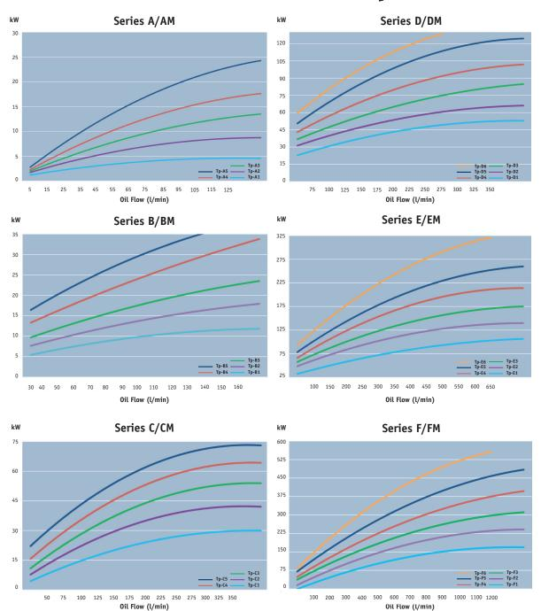
Graphs were plotted using the following parameters:  $\Delta T = 25$  °C, Viscosity of oil: 38 cSt (SAE 30) and water.
