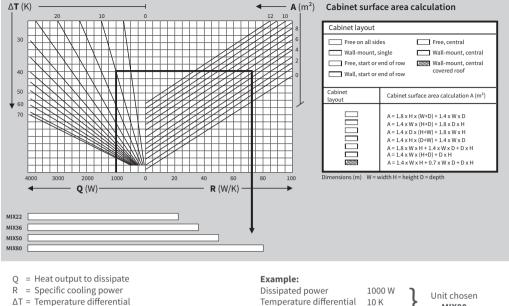
Temperature differential 10 K Cabinet surface area  $5 \text{ m}^2$
